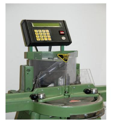
The autogage system (positoner) will allow the operator to make error-free movements.
